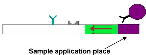
2) Addition of sample and analyte-specific solution
